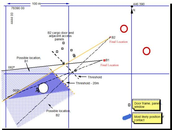
Figure 5: Debris trajectory analysis of cargo door parts from B1 and B2, indicating most likely location of impact.
