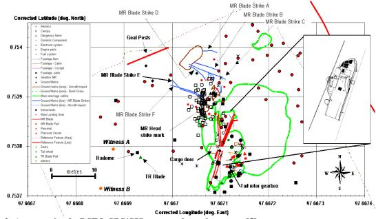
Figure 3: An example of a DSTO GPS/GIS generated wreckage map [5].
