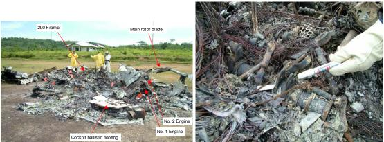
Figure 8. Sea King Accident Site, and disconnected fore/aft bellcrank (right)
