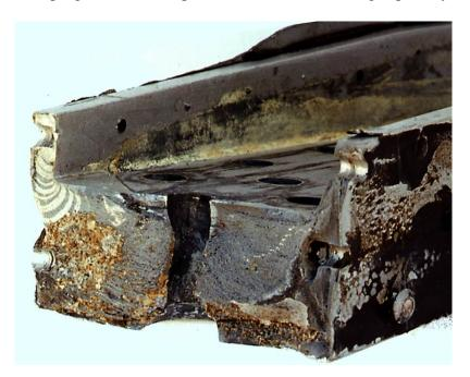
Figure 7: Fracture surface of A7-076 lower spar cap after recovery from the ocean. Note the fatigue progression marks propagating from the upper (nominally) blind fastener hole (upper left hand side).
