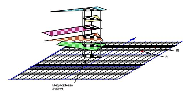
Figure 6: Most likely location of impact (grey shaded area). Each other colour represents the estimated projection of a component group (separated in height dimension for illustration purposes).
