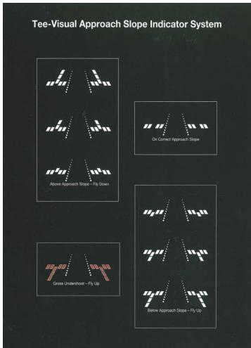
Figure 2: The Tee-Visual Approach Slope Indicator System runway light scheme
