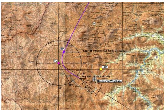
Figure 10: Reconstructed flight path showing approximate location of recovered aircraft. RP =Release Point, TL=Target Location, LKP= Last Known Position based on radar 1970. DSTO predicted quadrants including possible in-flight breakup (debris field based on fragmentation size).
